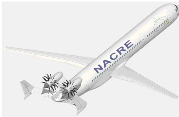
Fig. 1. A sustainable low-noise open-rotor-powered Pro-Green aircraft concept.
