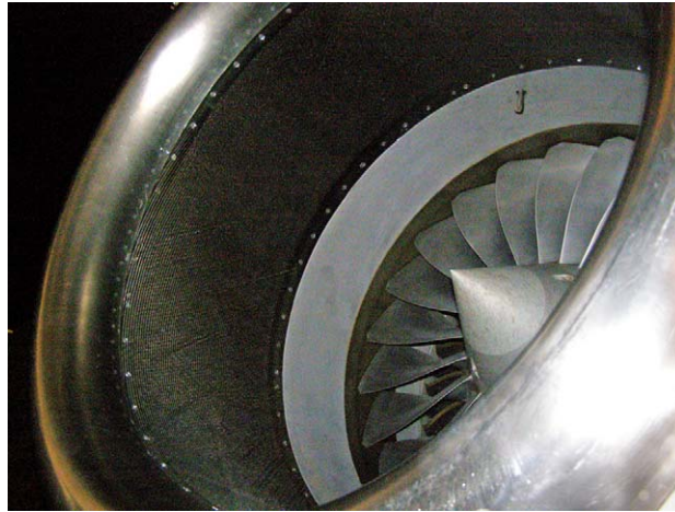
Fig. 32. Seamless double-layer intake acoustic liner.
